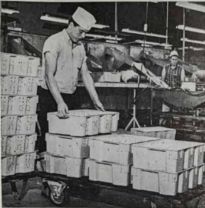
An important part of Mushroom Cooperative's freezing plant equipment is a grader (seen in background) that can grade in five size ranges with a tolerance of \frac{1}{4} inch.
