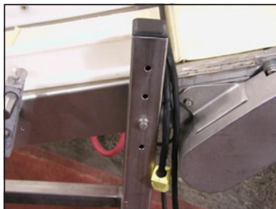
Seal holes in hollow frames and supports where moisture and Listeria can reside or, better, replace with solid supports.
