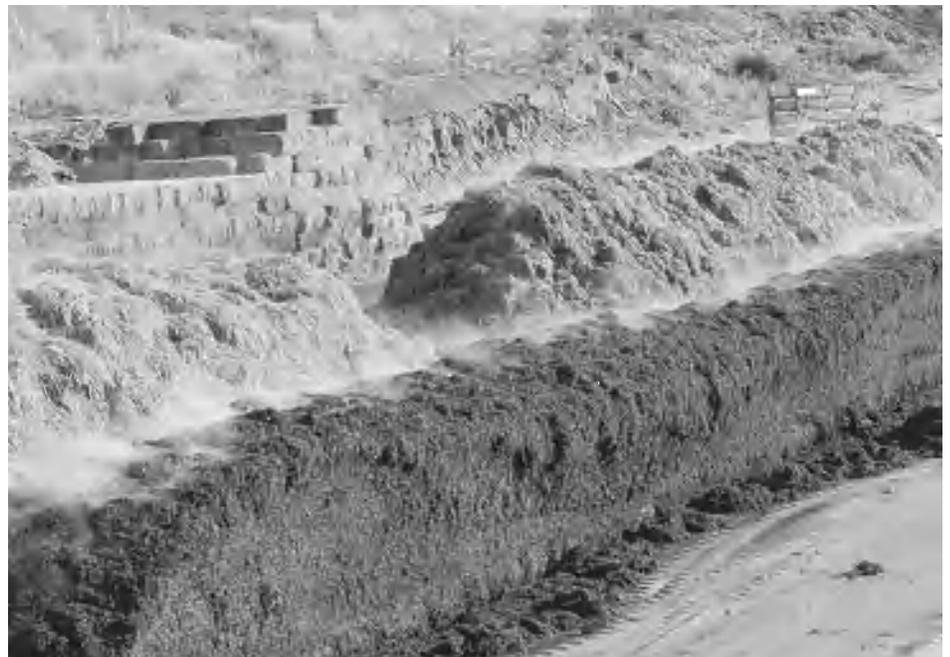
Figure 2 is a close-up of a machine “eating” its way through a compost pile. Once the pile is wetted and formed, aerobic fermentation (composting) commences as microbial growth and reproduction naturally occur in the bulk ingredients. Heat, ammonia, and carbon dioxide (CO<sub>2</sub>) are released as by-products during this process. Compost activators, other than those mentioned, are not needed.
