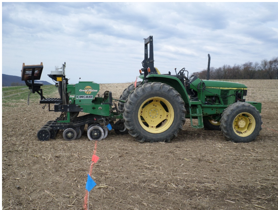
The MC was applied in 5' strips. A 5' Great Plains drill was used to plant a commercially available perennial grass mix and sorghum sudangrass for this experiment. (Planted May 1 st , 2015)
